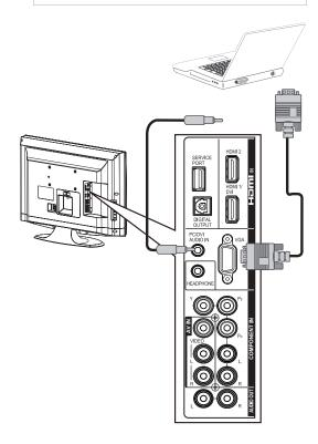
3 Connect an audio cable with stereo mini plug (not provided) to the PC/DVI AUDIO IN jack on the back of your TV and to the LINE OUT or AUDIO OUT jack on the computer.
